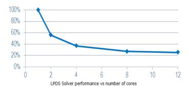
The most computationally intensive stages of the analysis using a sparse solver are generally decomposition of stiffness matrix and solving contact constraints. These are the stages which support multi-core, hence making them less time consuming.
